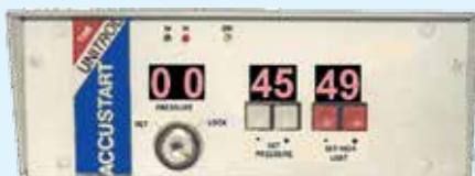
FIGURE 4: Stand-alone differential pressure transducer device that connects to an existing welding control can eliminate metal expulsion, improve weld strength, and increase electrode life.
