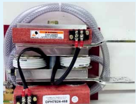
B. Direct-cooled SCR contactor with line voltage passing through the cooling hoses.
