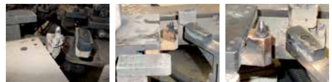
Ordinary MS resting / clamping block After 120 jobs & 160 m welding. AMPCOLOY® Mylar After 720 jobs & 958 m welding AMPCOLOY® Mylar After 4320 jobs & 5745 m
