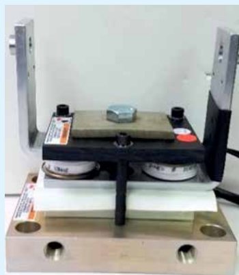
A. Indirect-cooled SCR contactor with no cooling hoses.
